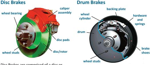
Disc Brakes are comprised of a disc or rotor, a caliper assembly, disc brake pads and the wheel bearings and hardware necessary to mount the components on the vehicle. The caliper is connected to the master cylinder through tubes, hoses and valves that conduct brake fluid through the system.
